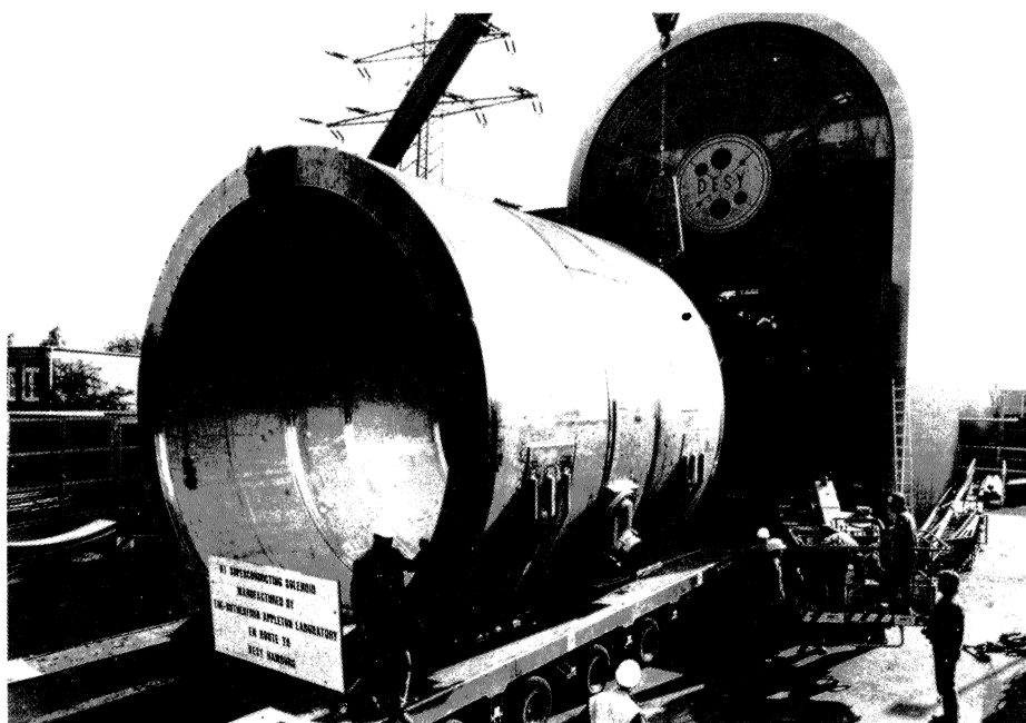
The superconducting coil manufactured by the UK Rutherford Appleton Laboratory for the H1 experiment arrives at the North Hall of the HERA electron-proton collider at DESY.
